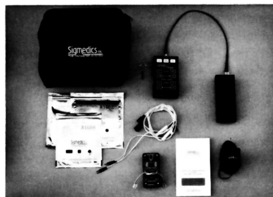
Figure 2. (Left) Someone using the system to stand. The battery and microprocessor are in the Parapack. Figure 3. (Below) The system including microprocessor, battery pack leader and surface electrodes.
